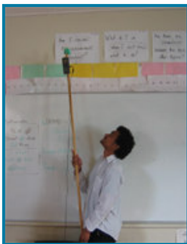
Student using sonic motion sensor to measure the speed of the balloon.
