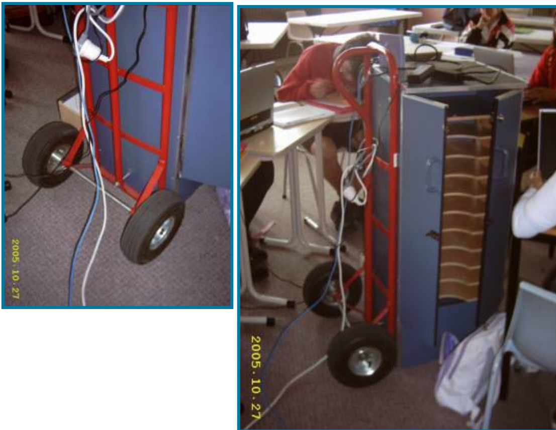
Figure 4: $40 truck from the local hardware store, bolted to the existing cabinet
